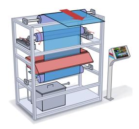
The Consultex Applicator can be used in conjunction with multi-device biax or blown-film lines; or, as a stand-alone offline coating system. Because of Its small footprint, it is easily retrofittable into existing lines. Turnkey systems also are available.
